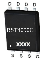
DFN5X6-8L top view
