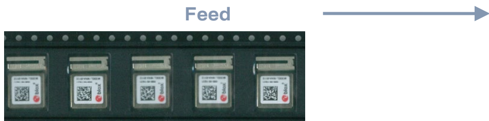
Figure 11: Orientation of NINA-B222 module on tape
