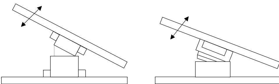
9. Keep the PCB warp 0.03mm or below as against the overall length of the connector.
