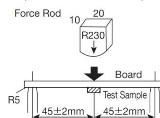
Printed board thickness: 1.0mm
