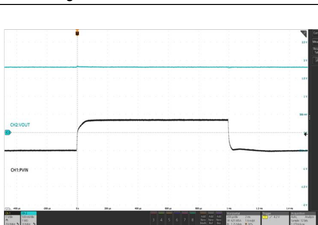
PV_{IN5} : 3.3V – 5V – 3.3V, V_{OUT5}=1.8\text{V} Figure 42. Buck 5 Line Transient
