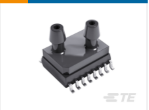
TE Part #9541-010C-D-C-3-S PRESSURE 0.15 PSID I2C SO16
