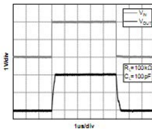
Figure 7. Large-Signal Step Response( V_S=5\text{V} )
