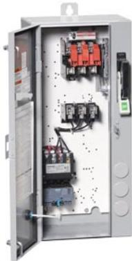
Non-reversing motor starter Size 1 Three phase full voltage Solid-state overload relay OLRelay amp range 0.75-3.4A 110-120/220-240VAC 60HZ coil Combination type 30Amp fusible disconnect 30 Amp /600V fuse clip Enclosure NEMA type 4/12 Water/dust tight weather proof Standard width enclosure
