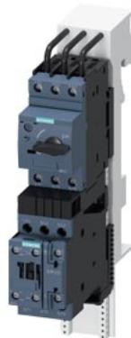
Fuseless motor starter Direct start 600VAC Size S0 2.8-4A 24V DC screw connection For snapping onto 60 mm busbar systems Type of coordination 2 IQ = 150 KA Also full fills type Of coordination 1 1NO+1NC (contactor)
