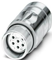
M23, Coupler connector, series: CA, straight, shielded: yes, for standard and SPEEDCON interlock, No. of pos.: 7, Direction of rotation: Standard, contact connection type: Socket, Solder connection, cable diameter range: 4 mm ... 6 mm, coding: N, Alternative product in accordance with RoHS II without Exemption 6c (Pb < 0.1 %) item no.: 1244031
