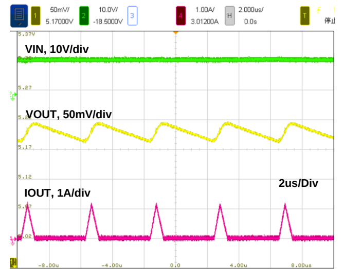
Figure 22. Switching Waveform, 100mA load
