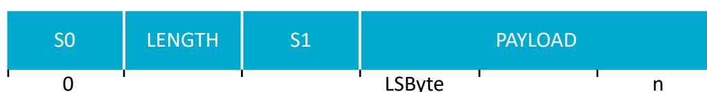
Figure 111: Representation of a RADIO packet in RAM
