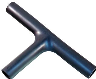
Low profile heat shrink “Tee” transitions provide an easy to repair and rugged cable routing solution. Transitional boots are available in eight material options with five adhesive choices. All Adhesive lined and unlined shrink boots are RoHS compliant. Transitional boots are water-tight when equipped with factory installed or user-installed adhesive. Choose boot size based on cable diameter.
