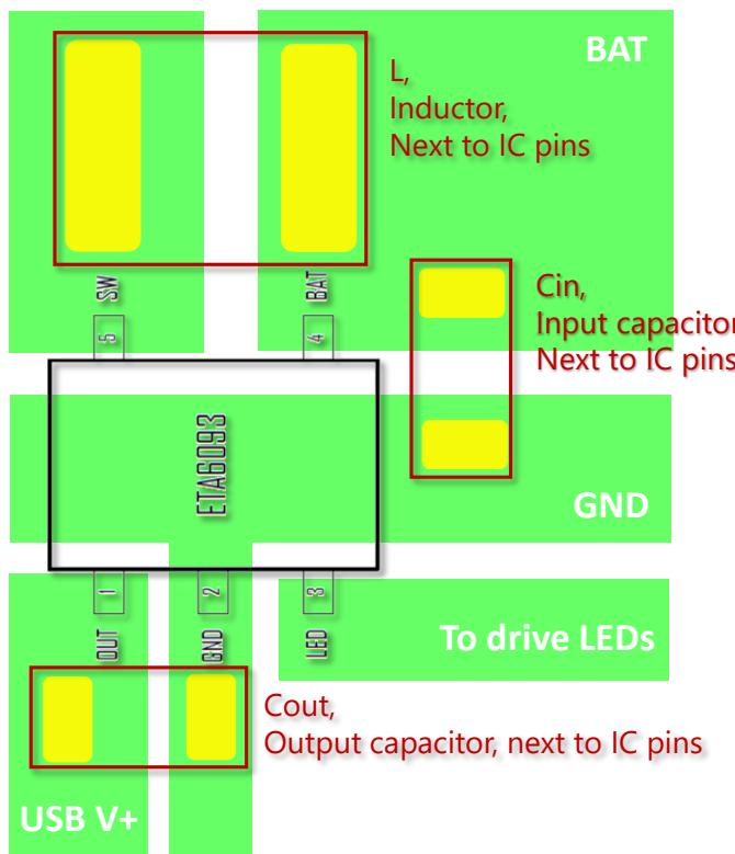
Please have the power devices placed just next to the IC pins so that the power traces are kept the shortest way to achieve a good performance of ETA6093.
