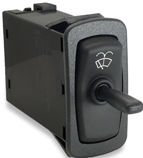
The LW-Series Electronic Wiper Washer Control combines two switches into one self-contained unit allowing effortless control of both wash and wipe functions from a singular location. A variety of features and options including, Continuous low and high speed wiper positions, Six intermittent delay intervals ranging from 3-18 seconds, Push-to-wash button and an LED Night-light indicator combine to provide the flexibility to meet most any Cab design.
