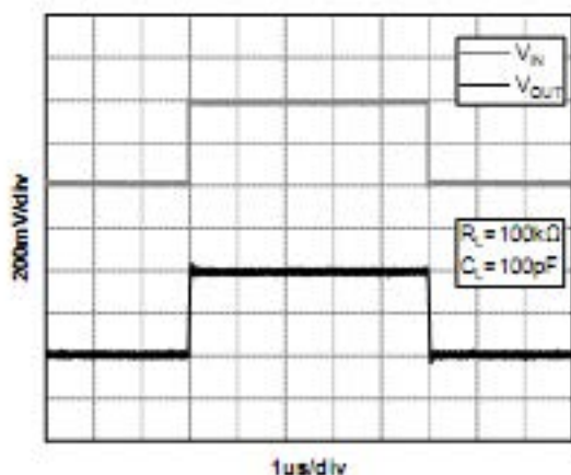
Figure 6. Small-Signal Step Response( V_S=5\text{V} )
