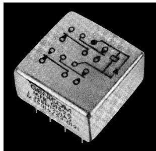
The 4PDT .150 Grid-space hybrid relays are advanced designs of the standard high reliability 4PDT .150 Grid-space relays. In the single diode version, the relay coil-back electromotive force is suppressed to prevent circuit/component damage. With the dual diode version, a steering diode is added to the coil circuit, along with the suppression diode. This
