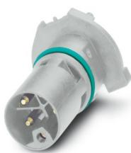
Contact carrier, Power, 5-position, Pin, straight, M12, coding: L, PCB mounting, THR solder connection, Item is lead-free in accordance with RoHS II without Exemption 6c (Pb < 0.1 %)
