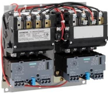
2-speed 3-phase motor starter Size 1 Two separate windings Constant or variable torque Solid-state overload relays Low SPD OLR range 3-12A High SPD OLR range 5.5-22A 110V 50HZ / 120V 60HZ coil Enclosure NEMA type (open) No enclosure
