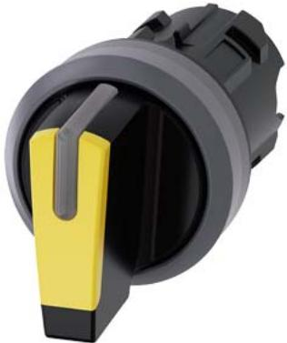
Selector switch, illuminable, 22 mm, round, plastic with metal front ring, yellow, selector switch, short, 3 switch positions I-O-II, latching, actuating angle 2x45°, 10:30h/12h/13:30h
