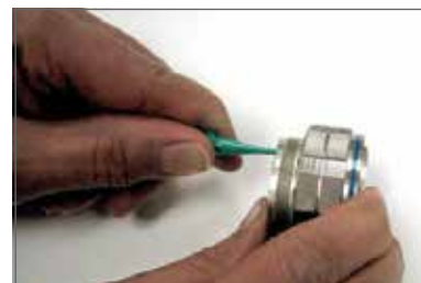
Plastic tool with contact in proper position.
