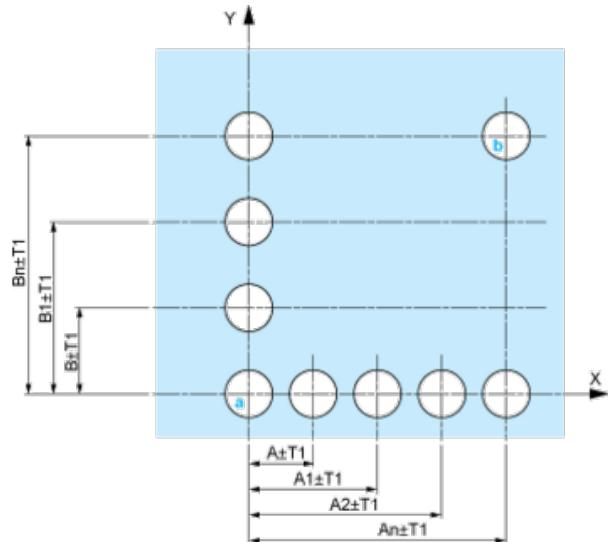
Printed Circuit Board Cut-outs (Viewed from Electrical Block Side)
