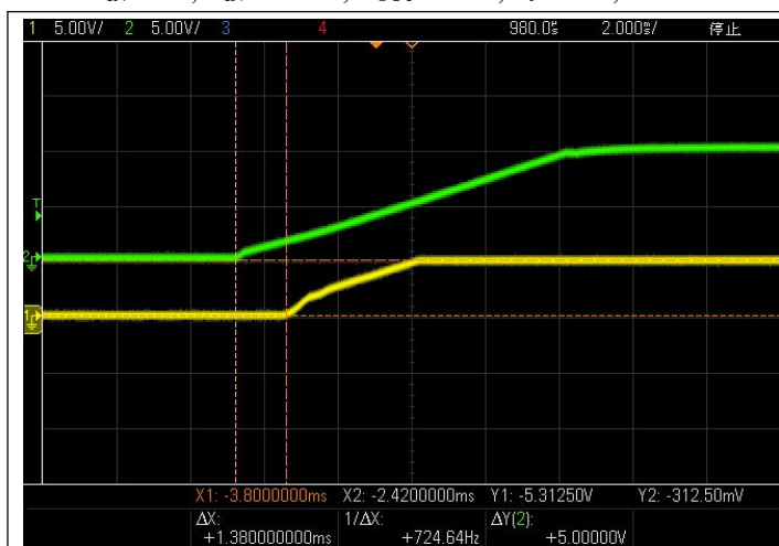
Fig 5. V_{IN} Start up ( I_{OUT}=0mA )
