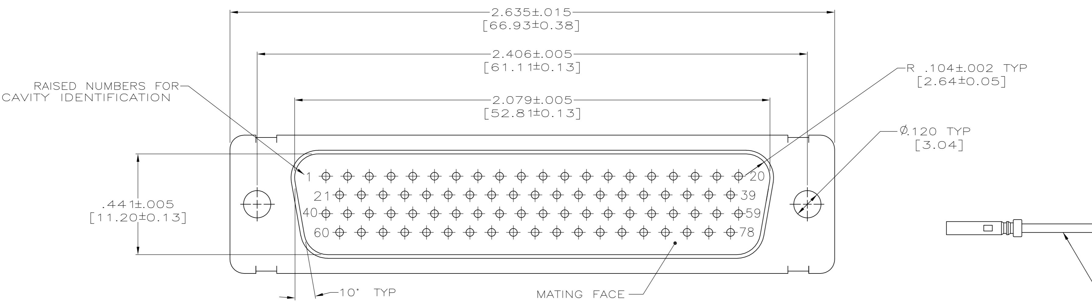
1. THIS PLUG WILL MATE WITH ANY SIZE 5, 78 POSN. RECEPTACLE IN AMPLIMITE SERIES.
