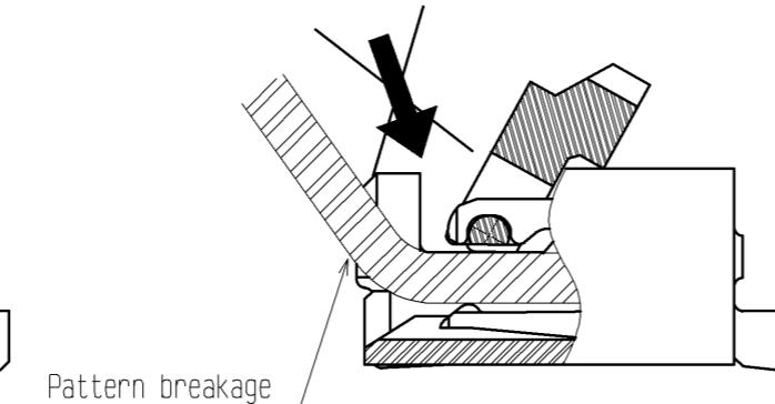
◆Checking the Locking Condition
