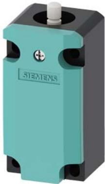
position switch basic switch plastic 40 mm according to EN 50041 increased corrosion protection device connection 1 x M20 x 1.5 1 NO/1 NC quick action contacts functional at -40 °C shock and vibration test according to DIN EN 61373, category 1B
