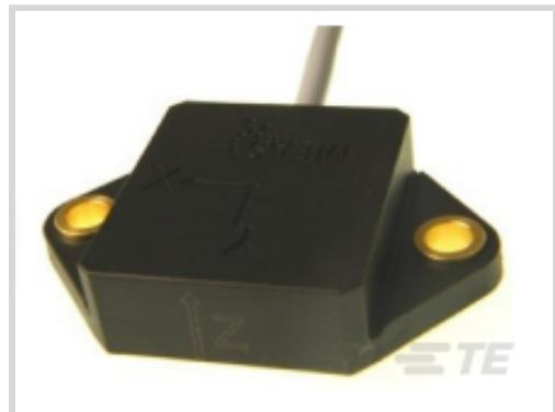
Accelerometer Type: **MEMS DC**Vibration Sensor Product Type: **MEMS Accelerometer**Number of Sensing Axes: **Triaxial**Frequency Response: **0-200 Hz**Full Scale Output Voltage: **.5 – 4.5 VDC**
