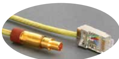
Quadrax Pin with 8P8C "RJ45" Jack
