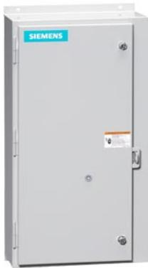
Non-reversing motor starter, Size 3 1/2, Three phase full voltage, Amb. compensate bimetal OLR, Contactor amp rating 115A, Non-combination type, Enclosure type 12, Dust/drip proof for indoors
