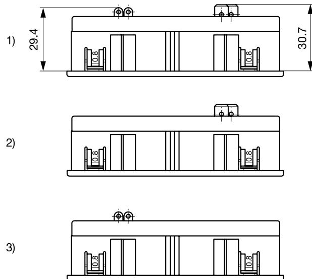
1) Solder and quick connect terminals 6.3x0.8 mm
