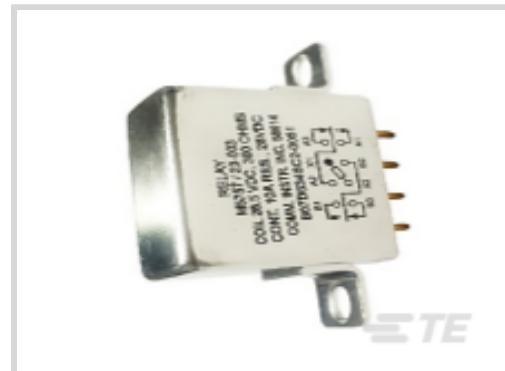
Relay & Contactor Type: **General Purpose Power Relay**Coil Magnetic System: **Non-Polarized, Monostable**Contact Arrangement: **2 Form C DPDT-CO**Current Type: **DC**Contact Current Rating: **10 A**
