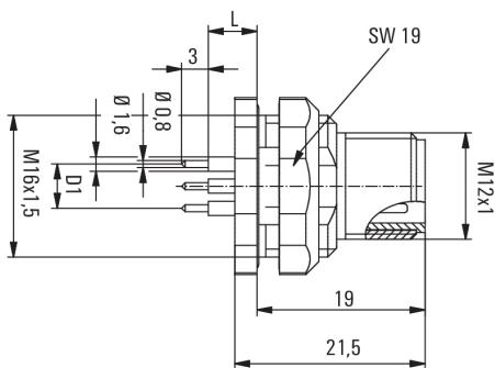
**Front panel section** D1 = 5,0 mm
