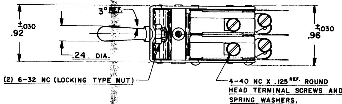
N.O. TO C. CIRCUIT MADE (SWITCH NO'S. 1 AND 2)
