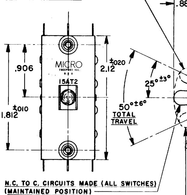
N.C. TO C. CIRCUITS MADE (ALL SWITCHES)
