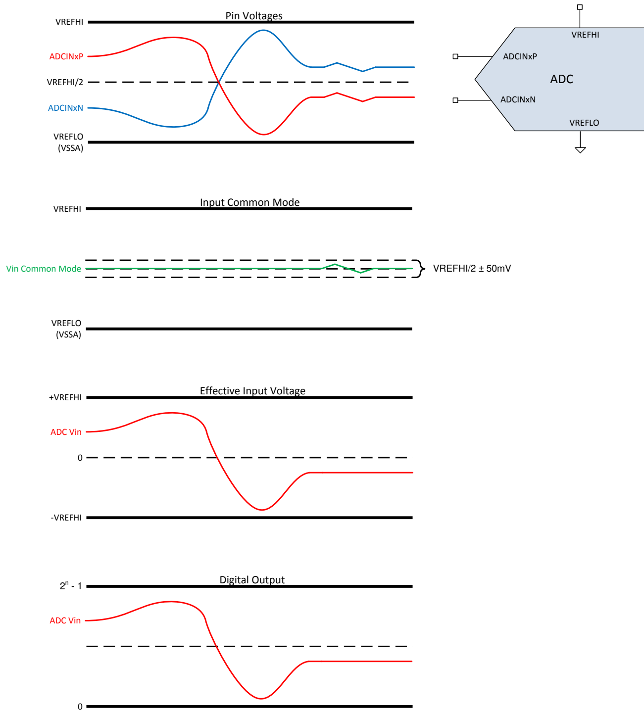
Figure 6-50. Differential Signaling Mode
