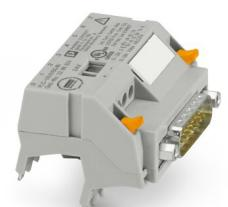
V8 adapter for 8 x PLC-INTERFACE (6.2 mm), controller: PLC system cabling of input cards, connection 1: D-SUB pin strip 1x 15-position, connection 2: Plug-in connection (Can be snapped onto 8x PLC-INTERFACE terminals), connection 3: Screw connection 1x 2-position, number of channels: 8, control logic: plusschaltend
