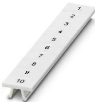
Zack marker strip, Strip, white, labeled, can be labeled with: CMS-P1-PLOTTER, Printed vertically: consecutive numbers 1 ... 10, 11 ... 20, etc. up to 491 ... 500, mounting type: snapped, for terminal block width: 6.2 mm, lettering field size: 6. 15 x 10.5 mm, Number of individual labels: 10
