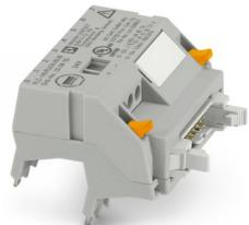
V8 adapter for 8 x PLC-INTERFACE (6.2 mm), controller: PLC system cabling of input cards, connection 1: IDC/FLK pin strip 1x 14-position, connection 2: Plug-in connection (Can be snapped onto 8x PLC-INTERFACE terminals), connection 3: Screw connection 1x 2-position, number of channels: 8, control logic: minusschaltend
