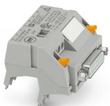
V8 adapter for 8 x PLC-INTERFACE (6.2 mm), controller: PLC system cabling of input cards, connection 1: D-SUB socket strip 1x 15-position, connection 2: Plug-in connection (Can be snapped onto 8x PLC-INTERFACE terminals), connection 3: Screw connection 1x 2-position, number of channels: 8, control logic: plusschaltend
