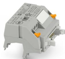
V8 adapter for 8 x PLC-INTERFACE (6.2 mm), controller: PLC system cabling of input cards, connection 1: IDC/FLK pin strip 1x 14-position, connection 2: Plug-in connection (Can be snapped onto 8x PLC-INTERFACE terminals), connection 3: Screw connection 1x 2-position, number of channels: 8, control logic: plusschaltend
