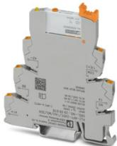
PLC-INTERFACE for input functions, consisting of PLC-BPT.../SEN basic terminal block with Push-in connection and plug-in miniature relay with multi-layer gold contact and manual operation, 1 N/O contact, 24 V DC input voltage
