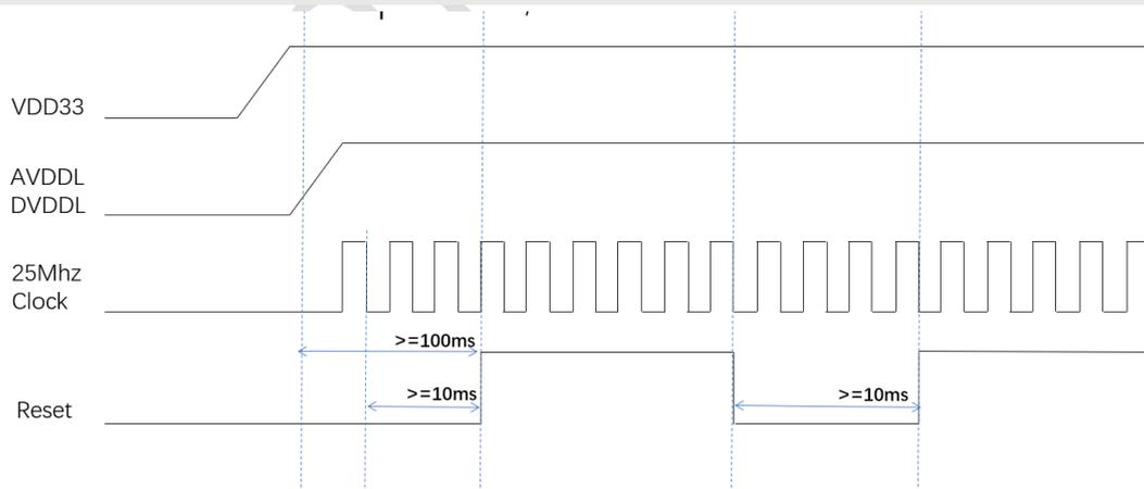
When using crystal, the clock is generated internally after power is stable. For a reliable power on reset, suggest to keep asserting the reset low long enough (100ms) to ensure the clock is stable and clock-to-reset 10ms requirement is satisfied.
