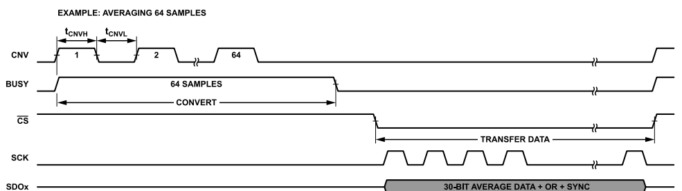
Figure 111. Example Conversion Cycle for Averaging Mode
