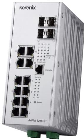
Korenix JetNet 5216GP Series, the DIN-Rail type industrial Gigabit Managed PoE Switch. JetNet 5216GP is the first industrial ethernet switch compliance with IEEE 802.3af/at/bt, each ethernet port can max supports 90W for PD, and total budget up to 480W <sup>\*Note</sup>.
