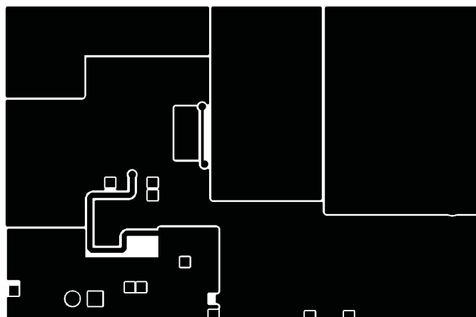
Figure 43. TPS40200EVM-001 Bottom Copper (X-Ray View From Top)
