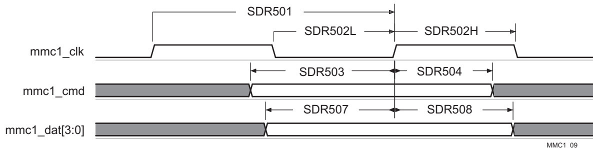
Figure 7-62. MMC/SD/SDIO in - High Speed SDR50 - Receiver Mode
