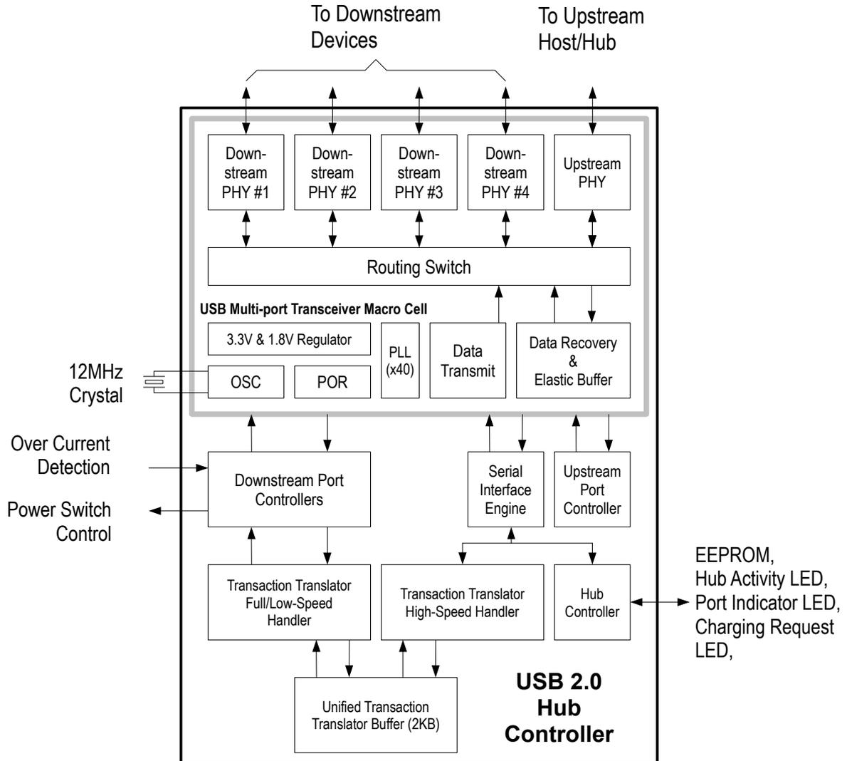
*Fig. 1: Block Diagram*
