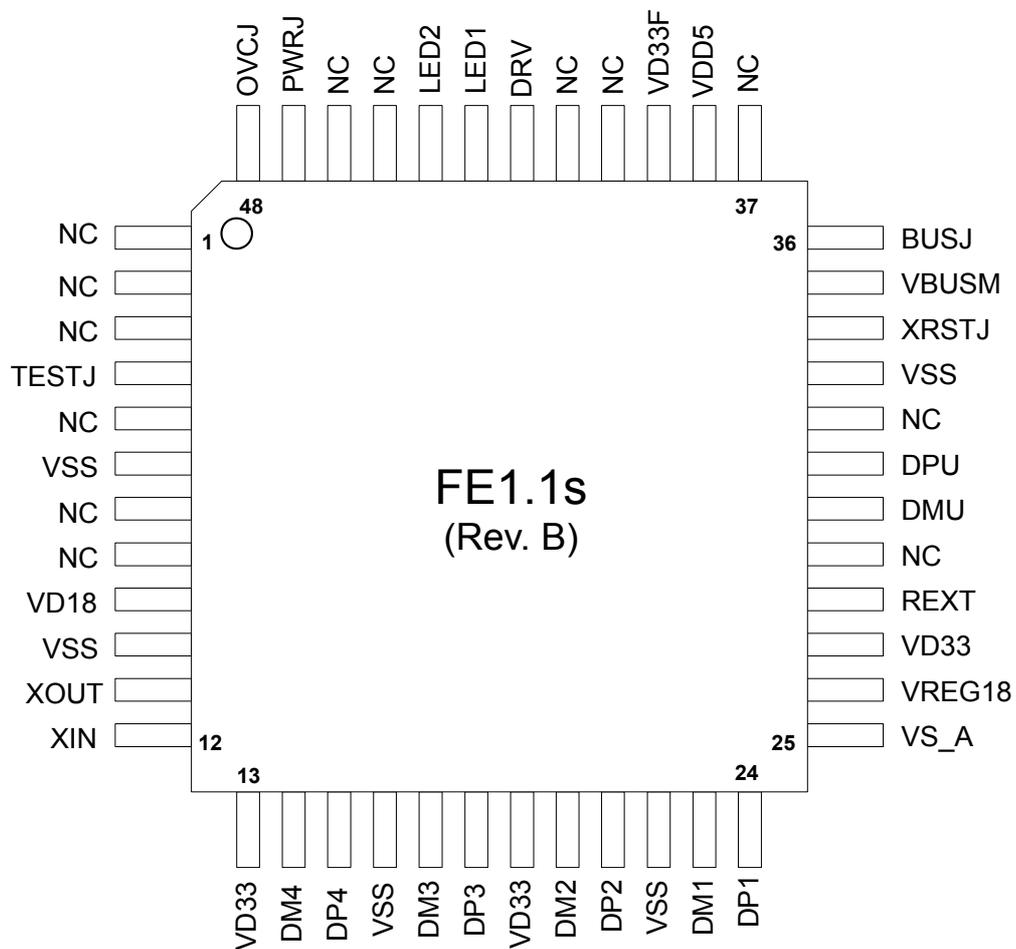
Fig. 4: 48-Pin LQFP Pin Assignment
