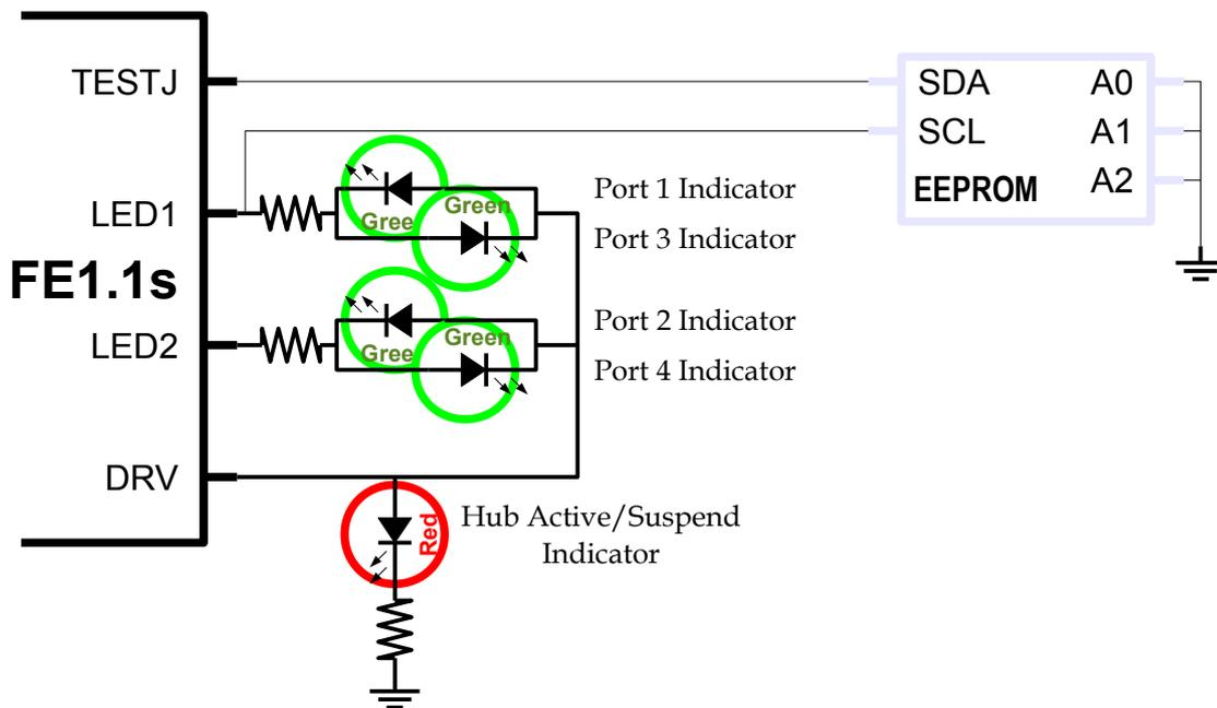
Fig. 5: Individual Port Indicator Configuration
