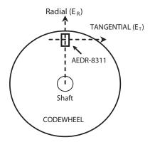
**Angular Misalignment Error (EA):** Angular displacement of the encoder relative to the tangential line.
