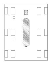
Note: The shaded areas are ⊠ not encoder pinouts. They ⊠ are electrically grounded ⊠ and physically exposed. ☒ PCB layout with tracks ☒ running across these areas ☒ should be avoided.
