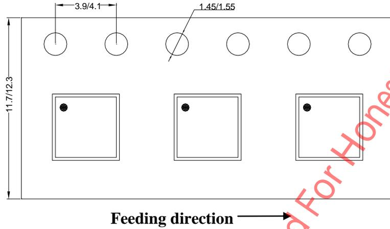
**2. Carrier Tape & Reel specification for packages**
