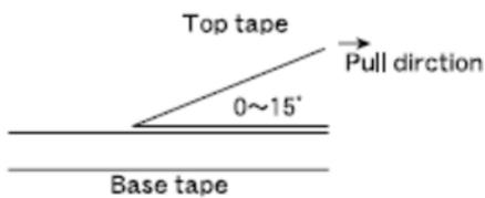
The top tape requires a peel-off force of 0.1 to 1.0N (0.315 inches wide) / 0.1 to 1.3N (0.472 inches wide) in the direction of the arrow as illustrated below.
