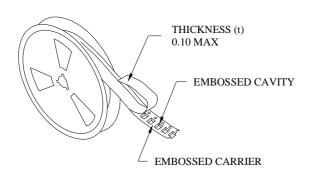
• THE FORCE FOR TEARING OFF COVER TAPE IS 10 TO 100 GRAMS IN THE ARROW DIRECTION.
