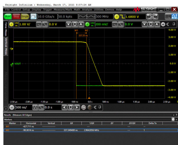
Figure 16. Overload Recovery at Positive Rail
