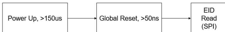
Figure 12 Pre-condition of EID Read
