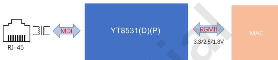
Figure 6. UTP<->RGMII Application Transmit Functions
