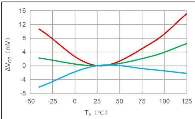
$\Delta V_{OE} \text{ vs } T_A$
