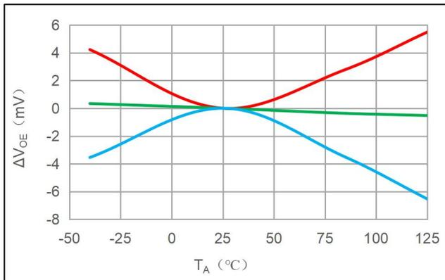
$\Delta V_{OE} \text{ vs } T_A$
