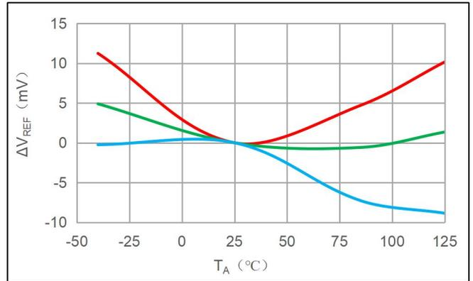
$\Delta V_{REF} \text{ vs } T_A$
