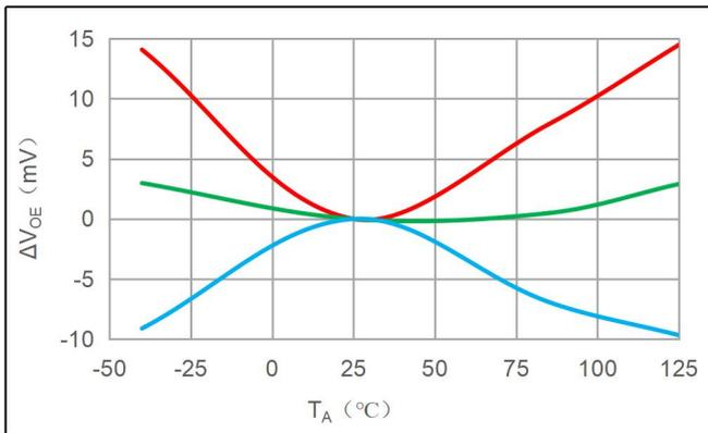
$\Delta V_{OE} \text{ vs } T_A$
