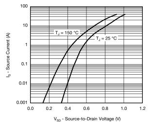
Source-Drain Diode Forward Voltage
