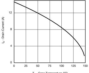
T<sub>C</sub> - Case Temperature (°C) **Current Derating\***
