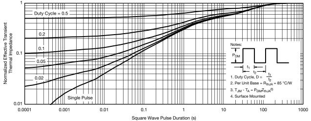
Normalized Thermal Transient Impedance, Junction-to-Ambient
