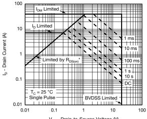
$V_{DS} \text{ - Drain-to-Source Voltage (V)} \\ ^*V_{GS} > \text{minimum } V_{GS} \text{ at which } R_{DS(on)} \text{ is specified} \\ \\ \text{ - One of the Descention A property of the Position A proper$
