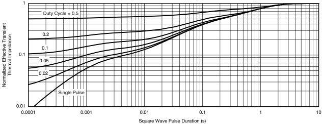
Normalized Thermal Transient Impedance, Junction-to-Foot
